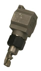
bearing grease. Place the nibbler head back onto the motor unit. Tighten the clamping screw snugly to lock the head assembly in place.
